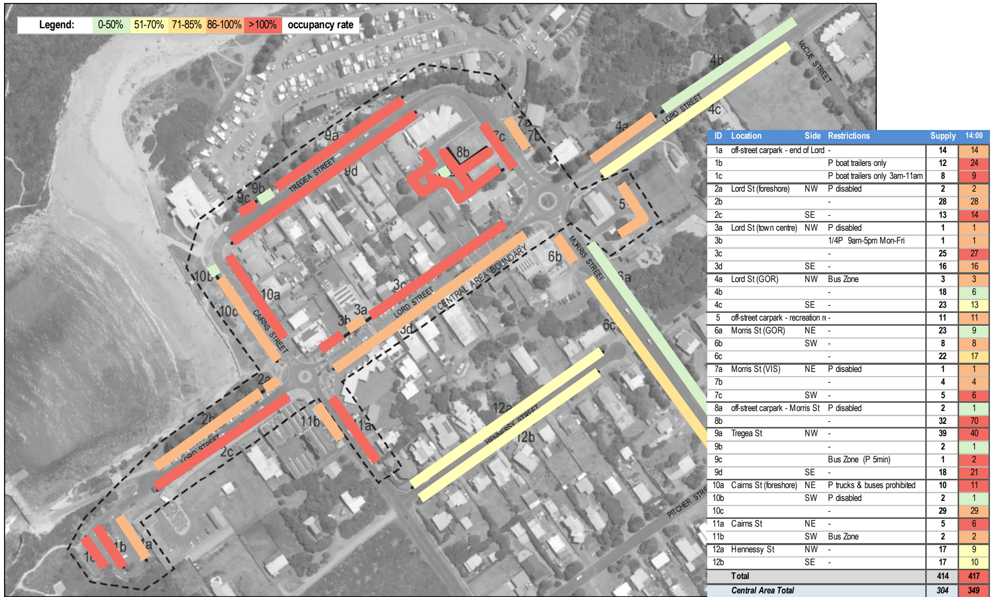
Figure 2.6 Peak Parking Occupancy Map on the Busiest Day (Saturday 28 th Dec. 2019 at 2:00pm)
