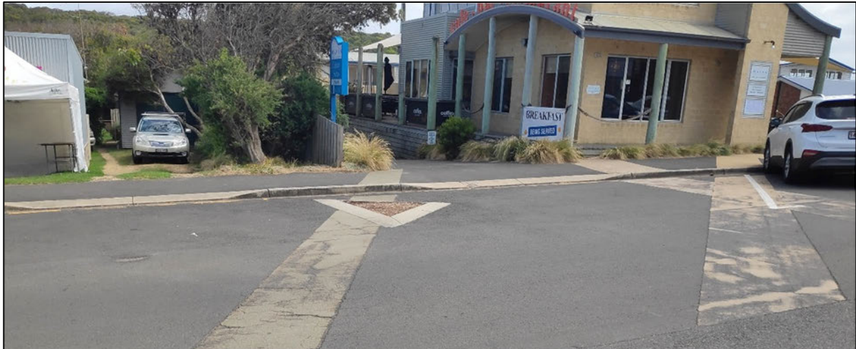
Figure 3.9 Example of Carriageway Area Not Intended as Parking Space but can be Utilised as a Space (also shows example of where motorcycle parking could be provided)
