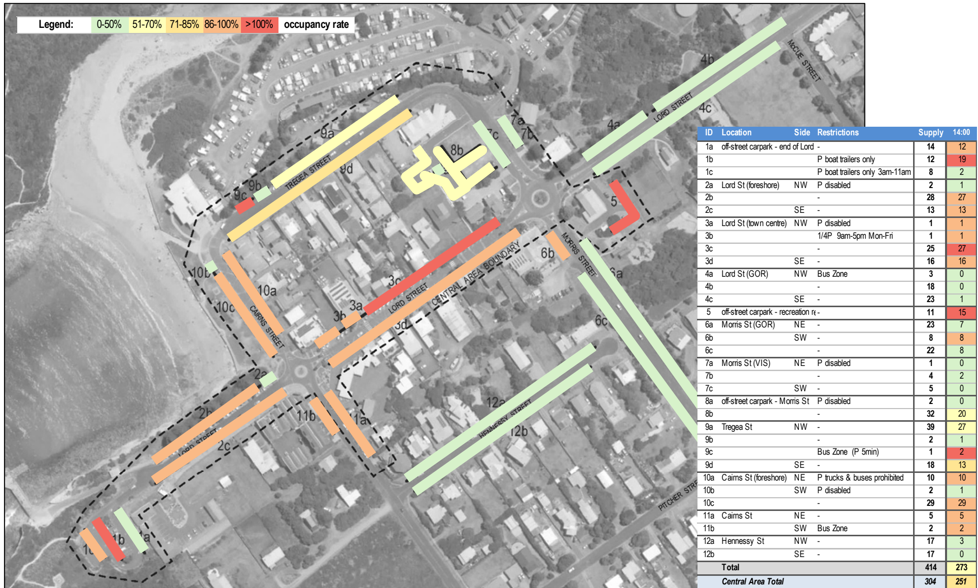
Figure 2.5 Peak Parking Occupancy Map on the Busiest Day (excl. Christmas / New Year) (Sunday, 26 th Jan. 2020 at 2:00pm)
